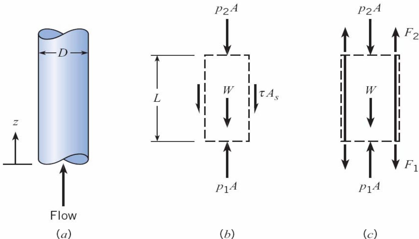
Forces associated with flow in a pipe: **(a)** pipe schematic, **(b)** control volume situated inside the pipe, and **(c)** control volume surrounding the pipe.
